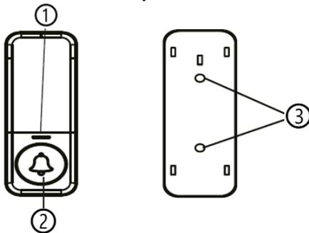
**The battery-free dynamo transmitter generates an electrical signal for ringing by converting mechanical energy at the push of a button. No need to worry about expensive battery replacements, especially in winter. Does not require special maintenance.**
